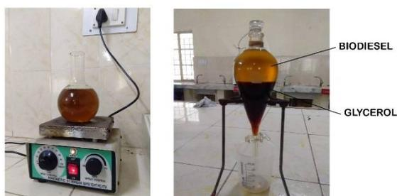
Fig 3.1: Heating of roselle oil Fig 3.2:Separating of Biodiesel
