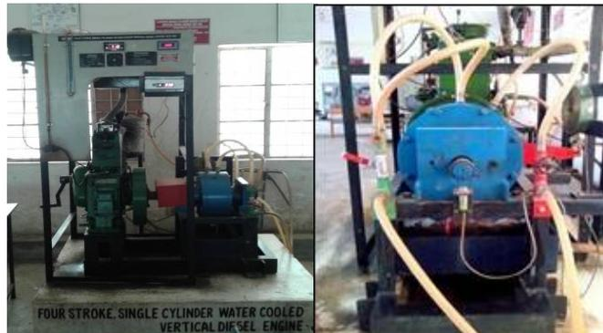
Fig 3.1: Diesel Engine
